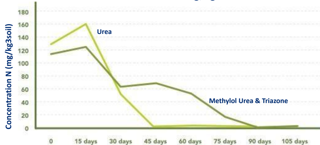
Ammonium release in a Webster soil (Iowa) Total N added 500mg/kg 3 soil
